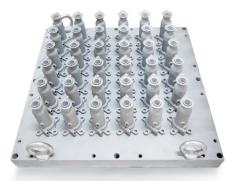
Multi-oil pipeline assembly parts IN718 high temperature alloy 420\*420\*110 mm<sup>3</sup>
