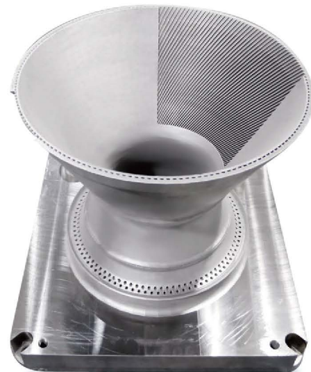
High quality large ejector cap with complex internal structures
